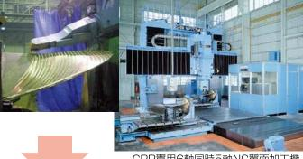
CPP翼用6軸同時5軸NC翼面加工機 6-axes with simultaneous 5-axes controlled NC blade milling machine for CPP
